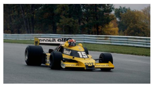
The option to run a turbocharged engine had been in the rules for many years, but nobody had dared to pursue it until Renault. It had quietly begun track testing with a 1.5-litre version of the turbo engine in 1976, and a short programme of races was scheduled for the following year.
